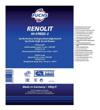
Our well proven grease RENOLIT HI-SPEED 2 gains more and more acceptance in applications like lubrication of high speed bearings in, e.g., machine tool spindles, and lubrication of linear guiding systems.
